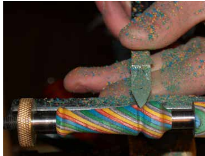
11 ... then switch to the hollower to form the bead as you'd like it, and to create a small decorative groove just below it
