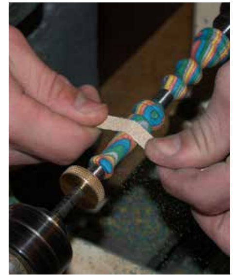
18 I like to work down from 120 grit to about 320 grit on pens
