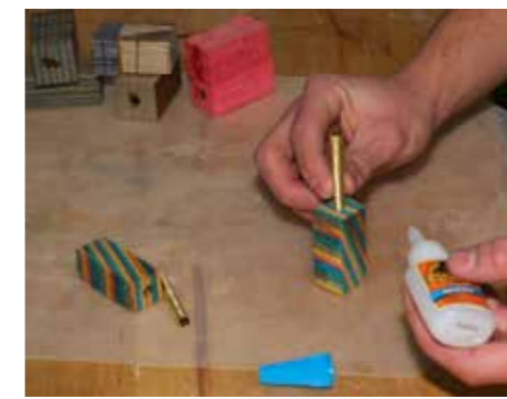
2 Secure the cylinders in the drilled holes with cyanoacrylate (CA) adhesive
