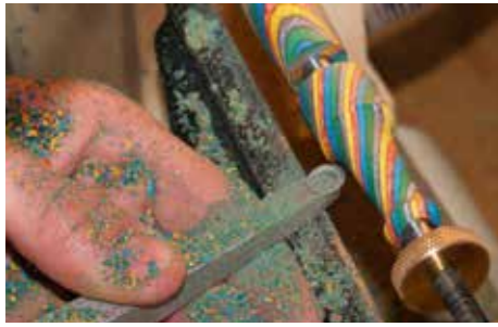
8 ... then create a gentle taper towards the centre of the pen, again using the round hollowing tool
