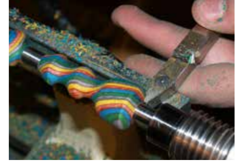
15 ... then switch to the detailer to fashion the head of the pen
