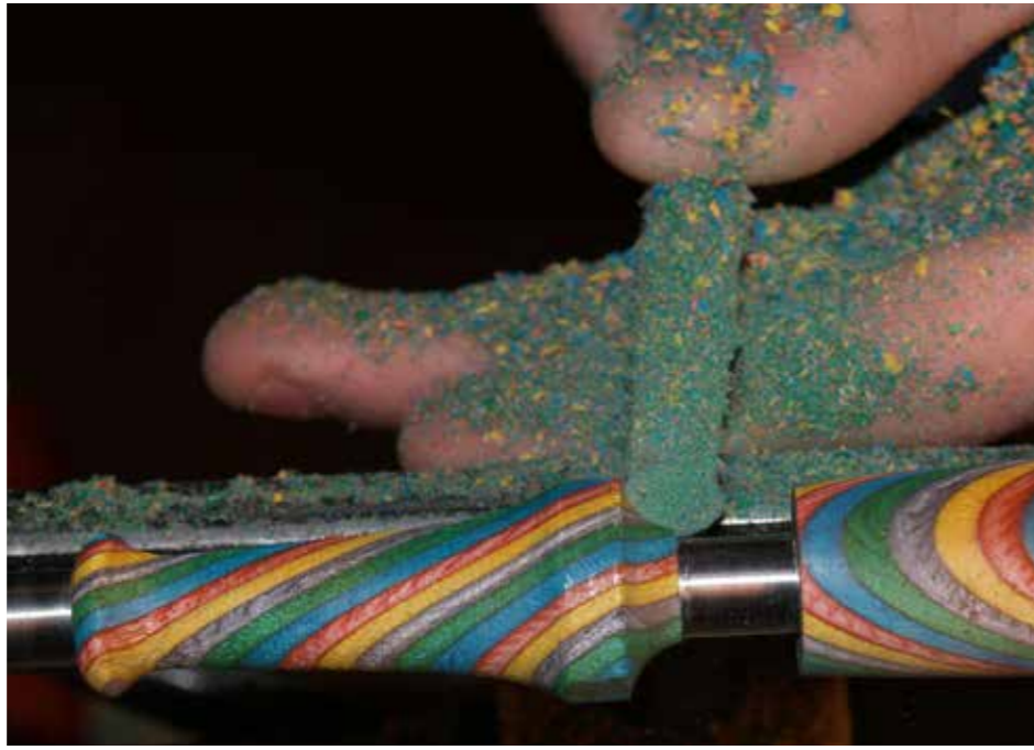
9 Create a cove that allows for a gracious transition from the wood to the metal bushing
