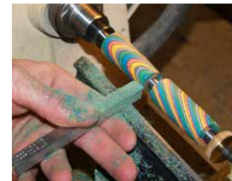
5 Reduce the blanks to round using the square cutter
