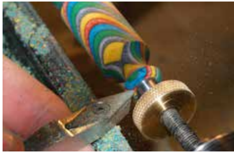
7 Clean up the bottom face of this latter curve using the point of the detailer...
