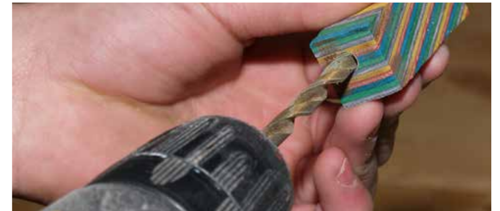
4 Use a drill bit to gently ream out the ends of the cylinders
