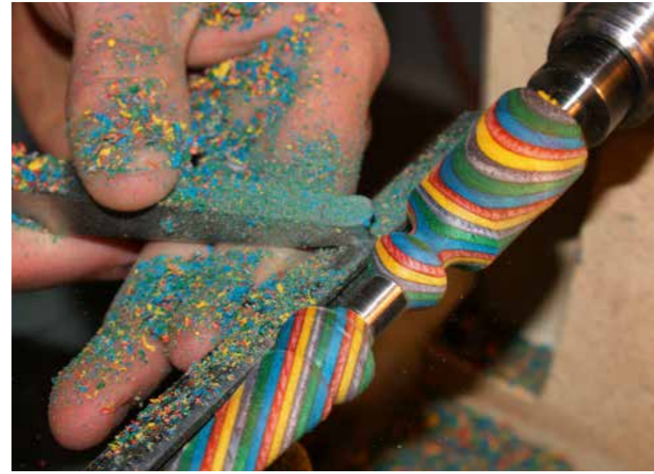
13 ... then stay with this tool to create a bead and a concave cove above this
