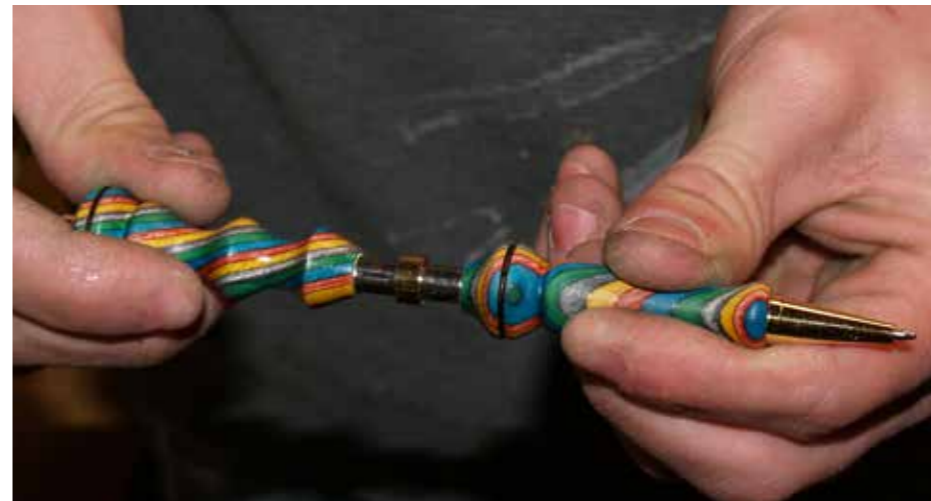
31 Slide the two parts of the pen together and the project is complete
