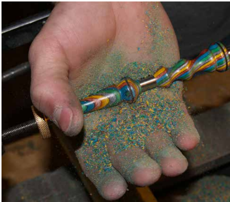
20 The shavings act like a mild abrasive and begin the polishing process
