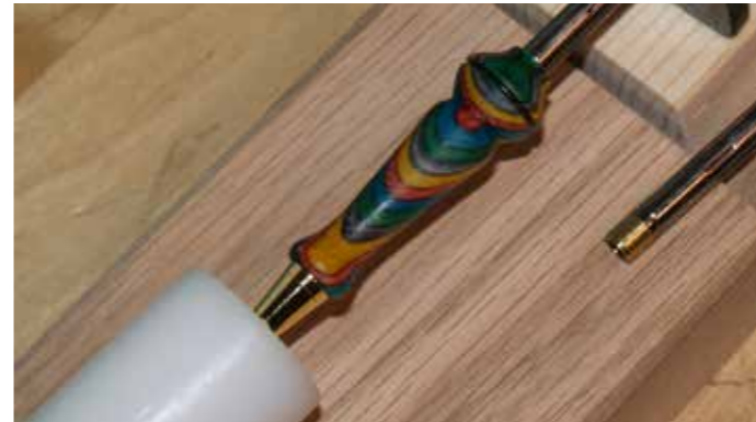
28 Push the cartridge into place, and test this as you go
