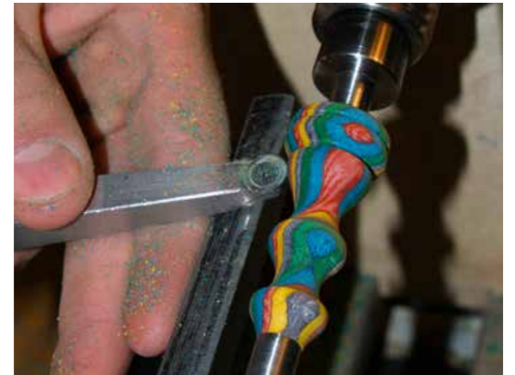
17 Smooth out the rest of the curves in a very light pass with the hollower
