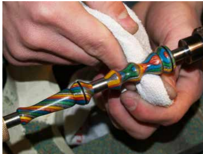
22 Polish this first coat of wax almost immediately at high speed
