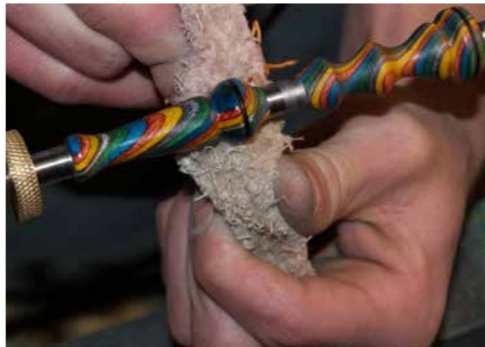
24 Wipe off the excess and then use the edge of a buffing wheel to polish the pen
