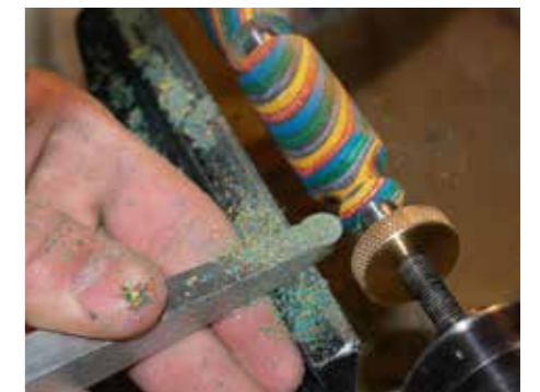
6 Use the hollower to create an inside (concave) curve where a writer's fingers will grip the pen
