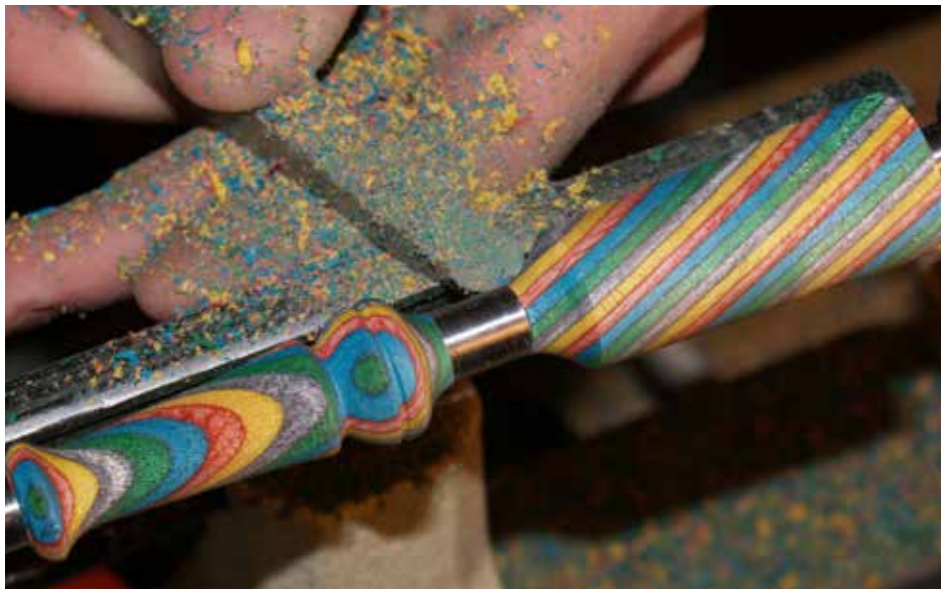
12 Use the hollower to make a matching cove at the bottom of the upper blank...
