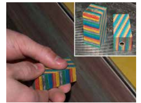
3 When dry, sand the ends of the blanks flush to the brass cylinders
